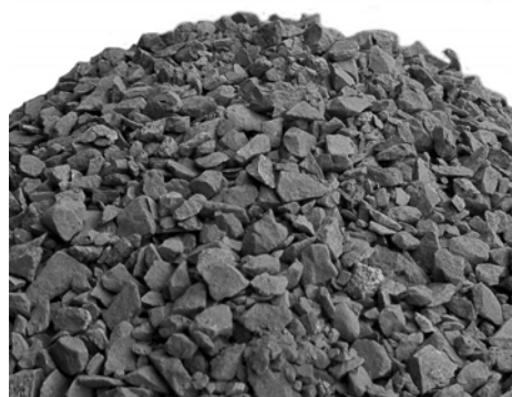
Mineral substrate as infill of drainage elements or as sub-substrate for intensive green roofs.
