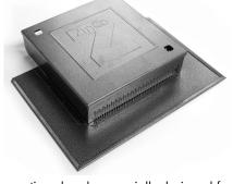
Made of galvanized and plastic-coated steel; with one side open and three sided flange, developed for water outlets near parapets or scuppers, can be used on fold-ups with insulation material fillet, perforated edges to install without tools. Detachable cover with two finger holes.
